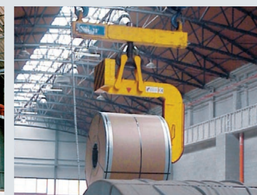
Bilanciere + gancio a "C" mod. 400+513 Lifting beam "C" mod. 400+513
